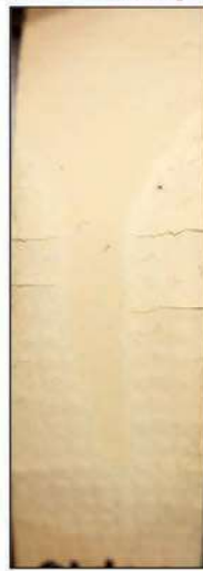
Figure 9 – Prior testing performed by René Dupuis illustrates the reason why we look at cracking of the membrane. The test sample is from laboratory exposure and the real-world sample is from an aged roof (not directly related to this study).
